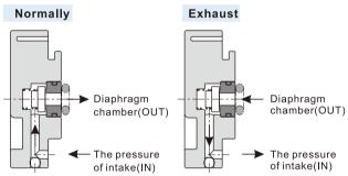
Normally, as the pressure of intake (IN) is higher than the set valve(pressure of outlet), the reverse flow valve closed; if the pressure of intake(IN) is cut off and starts exhaust, reverse flow valve opens. The pressure of diaphragm chamber is exhausted from IN orifice. At this moment, the pressure of diaphragm chamber decreases and the diaphragm is pressed down by the force from adjusting spring to open valve.
